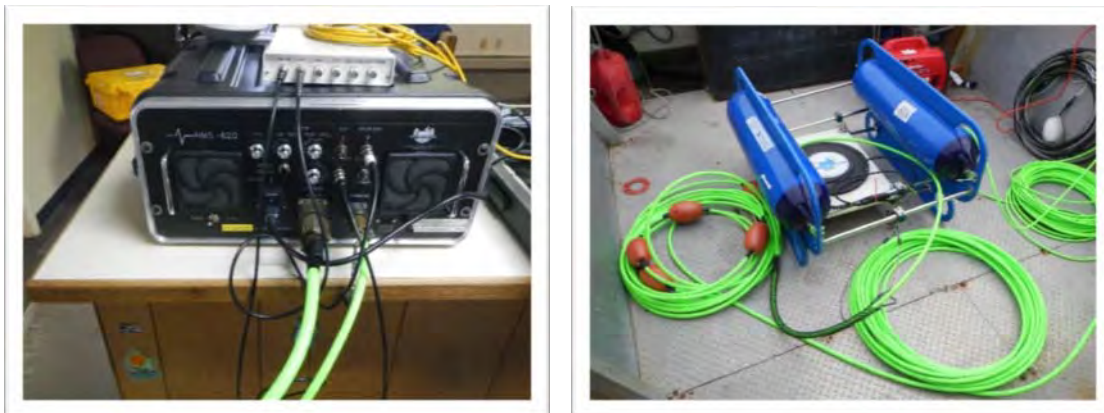
Figure 5. Falmouth Scientific Bubble Pulser. Acquisition system consisted of tow vehicle and transceiver.
