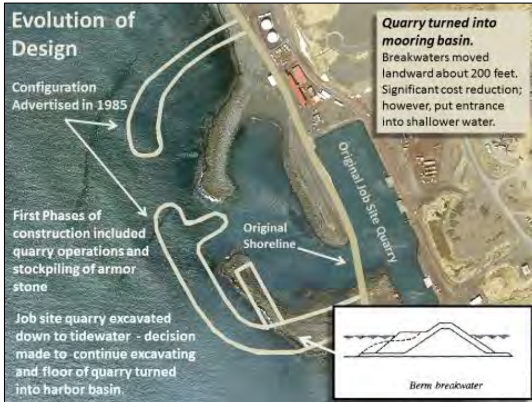
Figure C-4. Comparison of Constructed Harbor to Original Design (courtesy DOT&PF)
